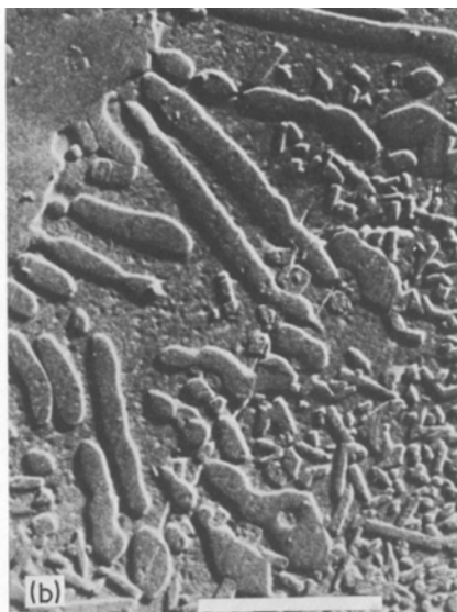
Figure 4 A TEM photograph showing the interface between the glass-ceramic (right side of each photograph) and the metal (left side of each photograph). The photograph in (b) is an enlargement of the rectangle in (a). Crystals in the bulk of glass-ceramic are below 0.5\ \mu\text{m} in size. Oriented larger crystals of about 1 to 2\ \mu\text{m} are grown along the interface. The white bar on the lower part of the right photograph indicates 1\ \mu\text{m} . Note a fracture propagated along the contact between the fine and coarse grain region, rather than along the contact between the glass-ceramic and the metal.
